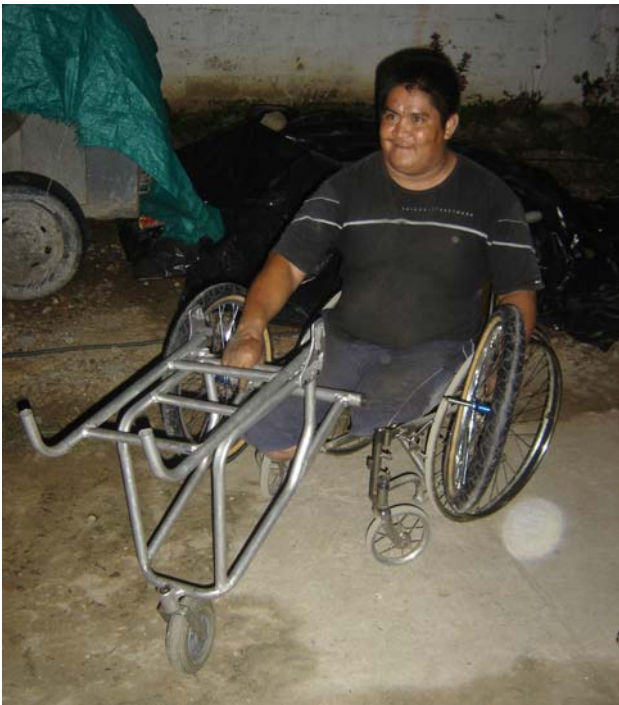
The stroller can be folded as demonstrated and the rear wheels can be easily detached. This package will fit into a trunk of a taxi. The chair will be detachable and will also fold to make it easy to carry. The detachable chair can also be used in the home if put into a rocking chair commonly found in homes.
