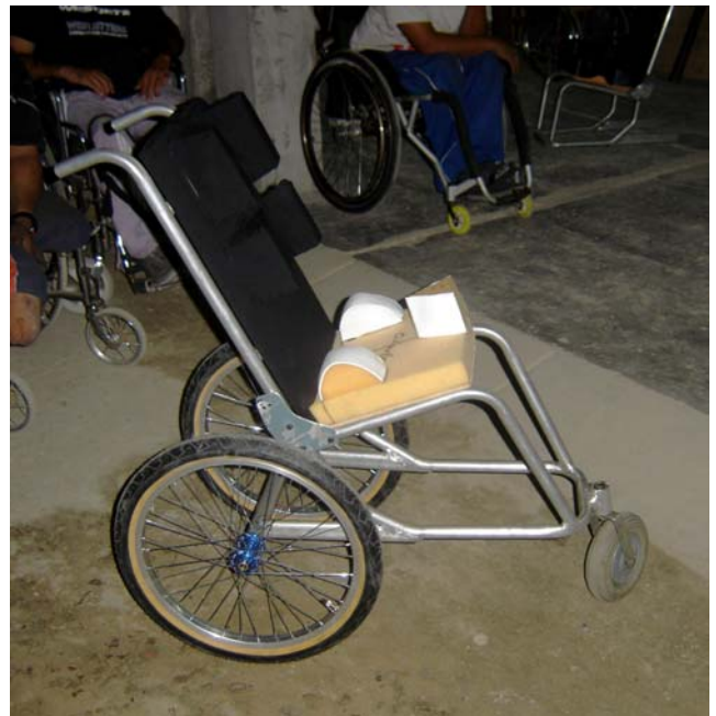
This is the stroller, still unfinished. It will be painted blue; side guards will be attached as well as a U hand-hold and a carrying bag at the base. I tested the stroller over very rough, rocky ground; it was light and easy to maneuver.
