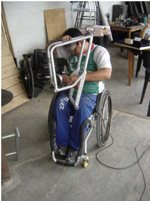
Ricardo, one of Jorge's assistants, is smoothing out the welds.
